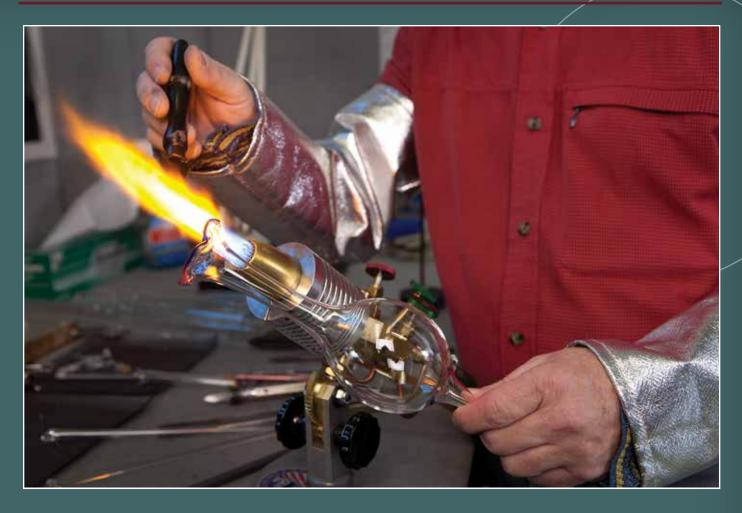
Smith makes a glass vase using a bench burner. The silver sleeves reflect the heat coming from the glass.
