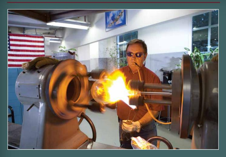
Smith repairs a recovery flask with the glass-blowing lathe in the university glass shop situated in Shelby Hall at the University of Alabama.
